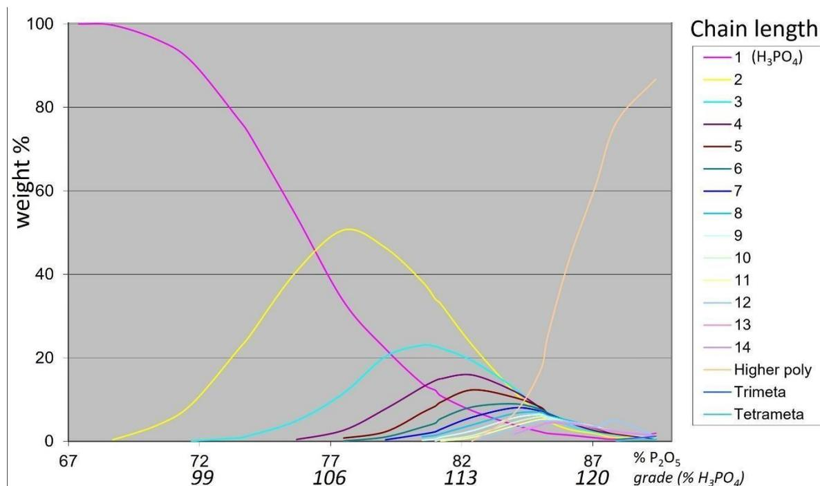
**Figure 14** Polyphosphoric acid chain length varies as a function of the  $P_2O_5$  content (% mass) and the grade number (%  $H_3PO_4$  by mass in solution), on the x-axis. Longer chain length implies more interlinked  $HPO_3$  units with  $PO_3H_2$  end groups. The chain length increases when the solution contains less water.
