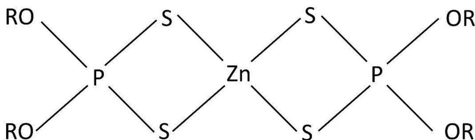
**Figure 30** Zinc dialkyl dithiophosphate (ZDDP) molecule. The bond structure around the Zn atom is indicative, it retains part of its 2+ charge and the two dithiophosphate units some of their negative charge. R denotes an organic group such as ethyl.
