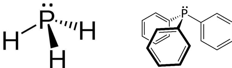
**Figure 32** Phosphine molecular structure. In the left panel, phosphine  $\text{PH}_3$ . Note the structural similarity of  $\text{PH}_3$  and  $\text{PCl}_3$ . The right panel illustrates triphenyl phosphine.
