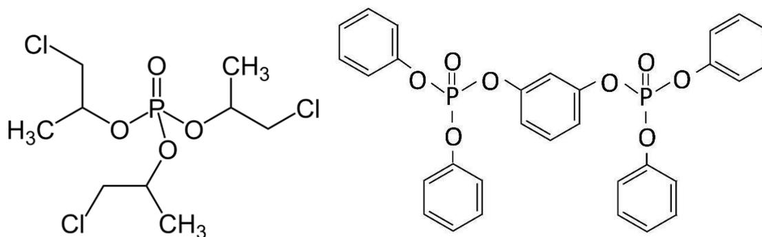
**Figure 25** TCPP (left) and RDP (right) molecule structures
