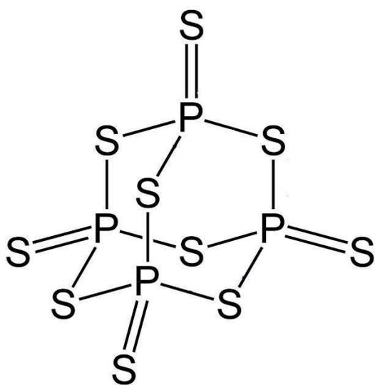
**Figure 27** The phosphorus sulphide (P<sub>4</sub>S<sub>10</sub>) molecule with an adamantane, cage-type structure.
