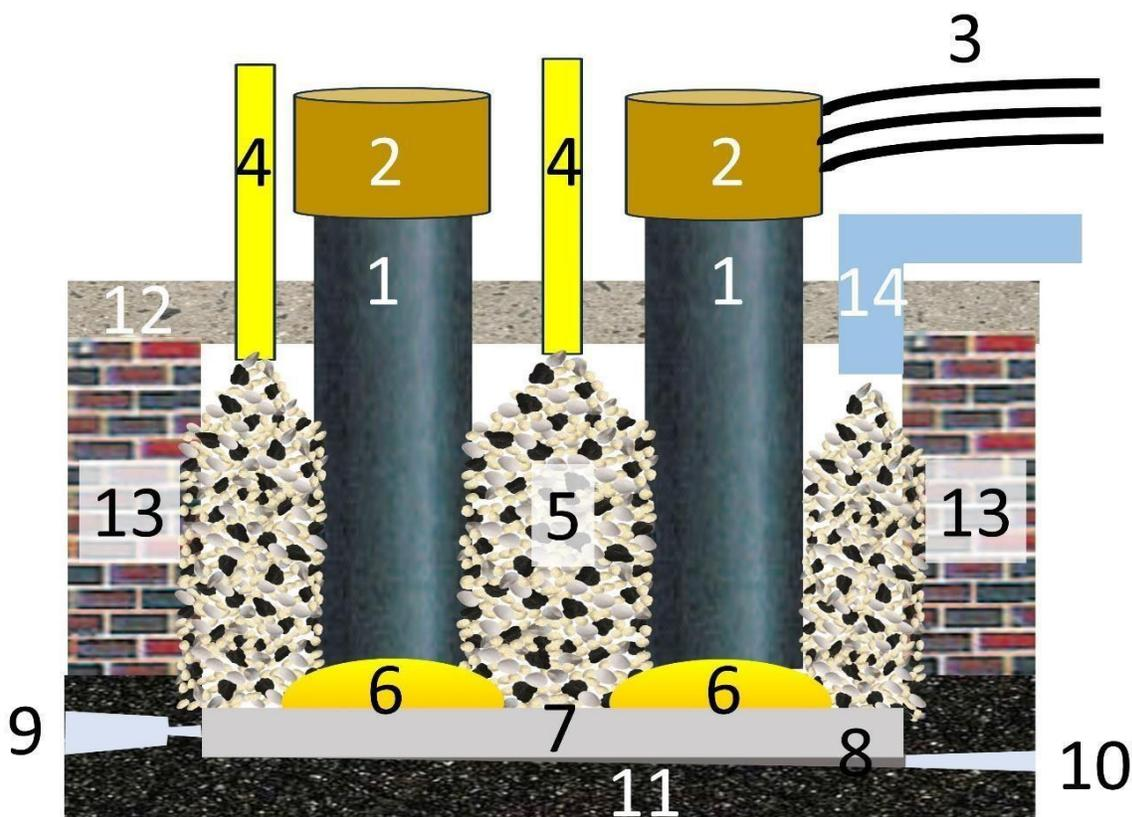
**Figure 4** Electrothermal reduction of rock phosphate is done in a submerged arc furnace.
